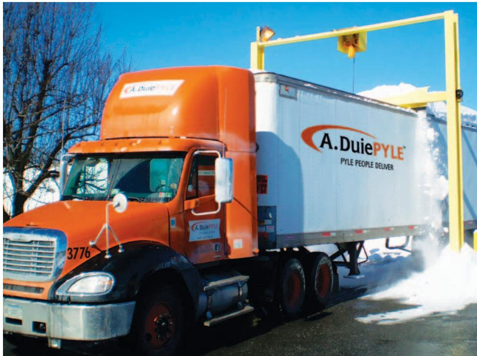
**The plow-like scraper removes snow as the trailer moves under the device. A rubber tip on the steel blade protects the roof. Pyle has 15 installed at its terminals in the Northeast, with two more scheduled.**
